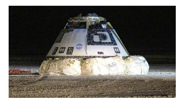
ILC Dover, LP produces the landing airbag and up-righting float systems for Boeing's CST-100 Starliner. *Credit: Boeing*
